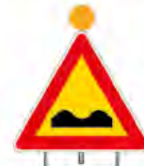
FIG. 389 ART. 31 STRADA DEFORMATA
